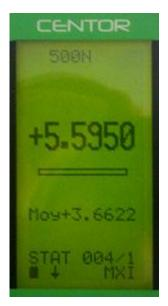
The measurement is performed by applying a torque to the pressure sensor ANDITORK. At any time the maximum is displayed in large characters on line 1. You can if you wish, display the current value instead of the maximum by pressing the top button (MAX).
